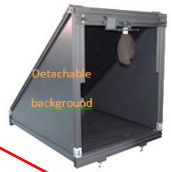
Detachable background panel and the threshold tool included in the software allows for easy background extraction
