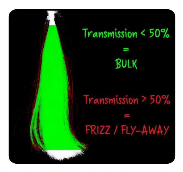
Once this separation between the bulk and the frizz / fly-away fibers is done, we can compute the ratio between those 2 components composing the hair fiber, to determine the increase or decrease in frizz.
