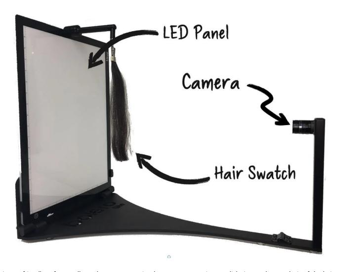
A user-friendly software allows the user to acquire the measurement in one click. A complete analysis of the hair swatch of the hair is delivered in seconds. Numerical data and images can be quickly compared and exported for reports, presentations or post processing.
