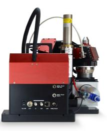
For measuring the caustic of a focused laser, the internal axes are moving the complete optical setup along the propagation of the laser. With its optional mount for fiber sockets, it is possible to measure the influence of a focusing head on a fiber laser with the MSM+ HB.
