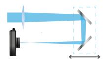
Inside the BEAMAGE-M2, a computer-controlled motorized rail allows precise positioning of two mirrors, which in turn allow a 400 mm beam path difference. At each position of the translation stage, a beam profile is acquired and the beam diameter is measured. The automation of the translation stage allowed by the software is the key to a fast measurement.
