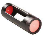
Each BEAMAGE-M2 system includes an alignment tube that helps you set up the system faster. Simply use the two alignment mirrors to center your laser beam onto both irises, and you will be ready to start measuring in no time!
