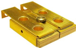
This Linear stacked Array "L2" type is an association of two stacks with 2 X 'zz' bars per stack. 'zz' can be 2 to 12 diode bars which gives stacks of 4 to 24 diode bars.
