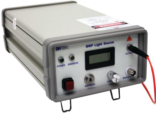
With up to 450mW of continuous laser power, the BWF1 is a fully integrated turnkey laser solution. The BWF1 is built to include features such as an external TTL modulation port (BNC connector) and an LCD display for setting laser power.
